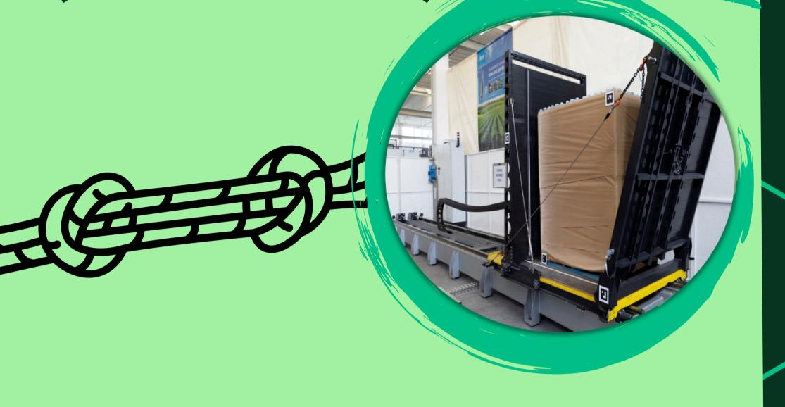
Acceleration test results showed that a pallet wrapped with kraft paper exhibits less deformation than the same pallet wrapped with stretch film.
